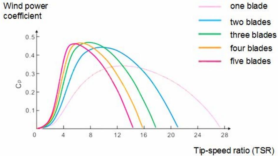
The power coefficient is a measure of how efficiently the wind turbine converts energy in the wind into electricity. Data is obtained by dividing the electricity produced by the turbine by the total energy available in the wind. Therefore a high power coefficient indicates a high efficiency at a certain wind speed.
